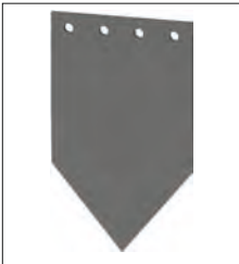
334.001.3: V-shaped knife. Standard blade for the UPG 10 Universal knife, usable for most thin-walled industrial hose assemblies with/without plastic spiral. Not suitable for hoses with steel reinforcement
