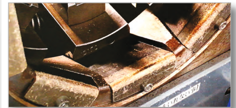
Sliding bearing in condition after ca. 900.000 crimping operations
