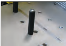
Guide pins ensure straight cuts.
