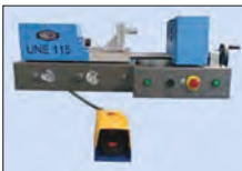
Preloading Safety control coupled to foot pedal.
