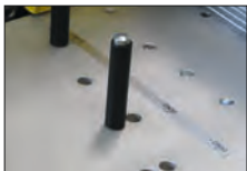
Guide pins ensure straight cuts.
