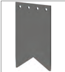
334.033.4: A-fine knife. Accessories UPG 10. For very soft hose assemblies with thicker wall thickness, e.g. rubber hose assemblies. Not suitable for hoses with steel reinforcement
