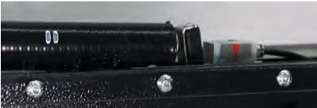
UNIFLEX insert – marking tool (ferrule position marking increases productivity and improves safety in hose sizes up to 2".
