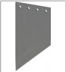
334.034.4: \-shaped knife (sloping). Accessory UPG 10. For hose assemblies without spiral with thin to thick wall thickness. Prevents deformation of the hose line during cutting = very straight cut.
