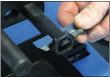
Skiving mandrels are manually adjustable.
