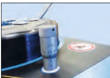
The micrometer allows you to easily set the crimping dimensions.
